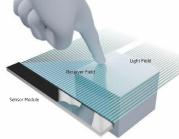
Neonode zForce (Zero-Force) optical reflective platform is based on light reflection technology, integrating optics and electronics in a thin strip along one side of an intended interactive area, creating a 2-dimensional interactive plane.
